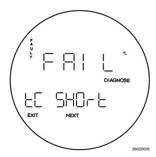
Figure 6-7. Fault 3, Shorted Thermocouple
